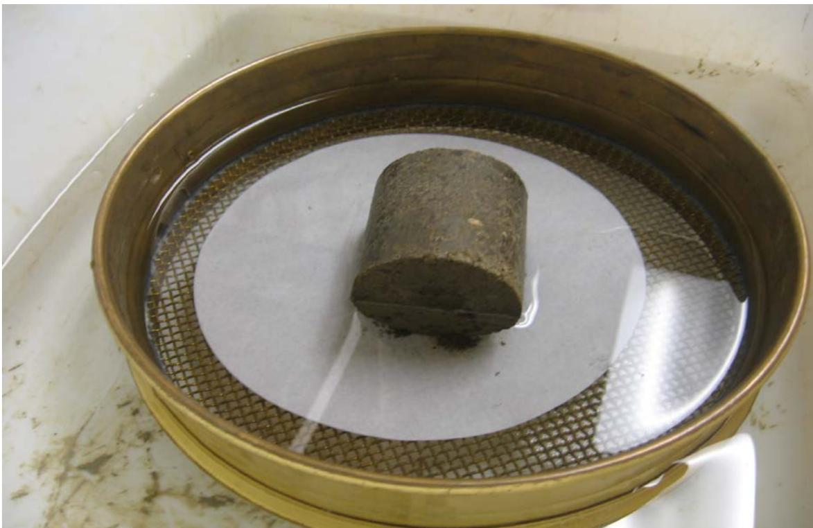
**Fig. 1.** Example of fly ash treated specimen under half saturation procedure
