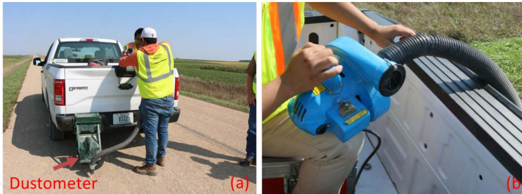
Figure 4. Installing the (a) dustometer device and (b) vacuum pump.
