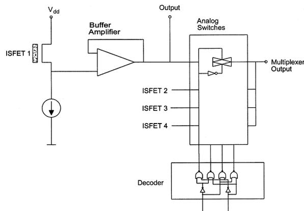
Fig. 1. Circuit diagram of the integrated multi-ISFET chip.
