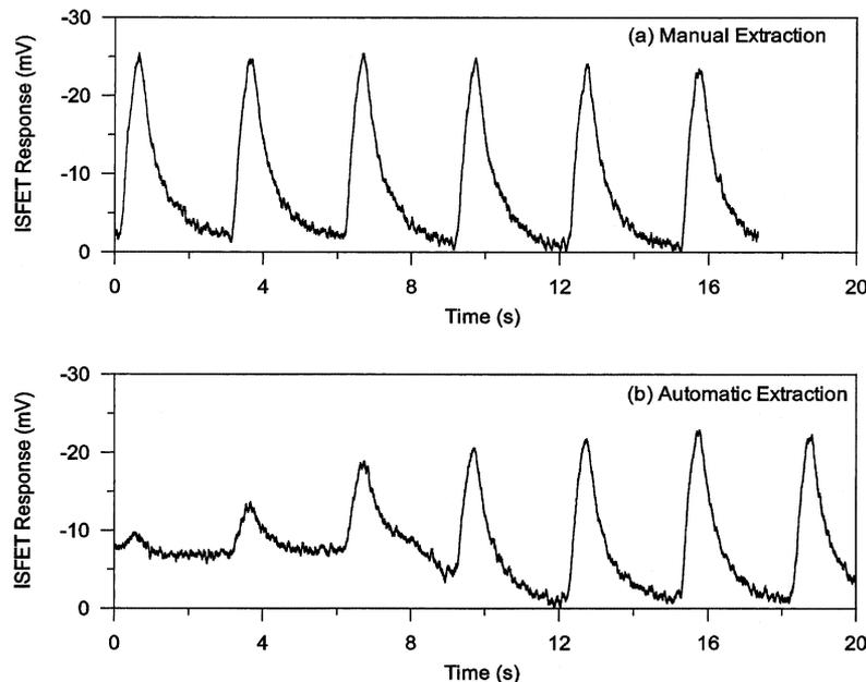
Fig. 8. ISFET response to (a) injection of manually extracted soil solution, and (b) injection of soil solution from the automated soil extraction system.
