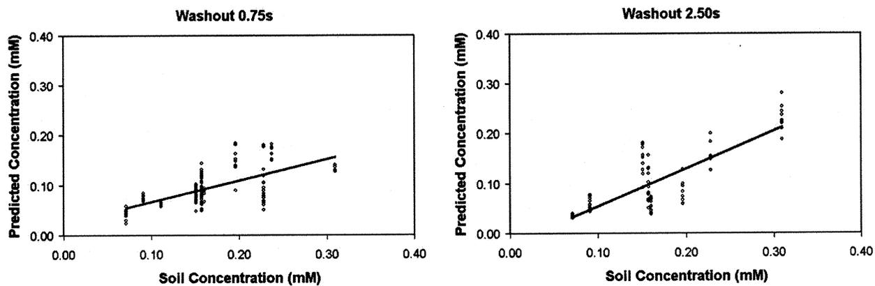
Fig. 9. ISFET/FIA predicted concentration for automatically extracted samples vs. actual soil nitrate concentration from manually extracted solutions, with 0.75 s (left) and 2.5 s (right) washout time.
