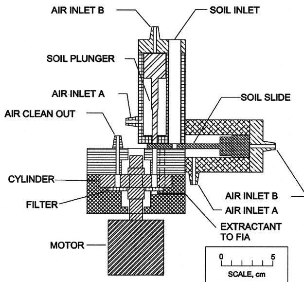
Fig. 3. Modified cross-section of automated extraction system.
