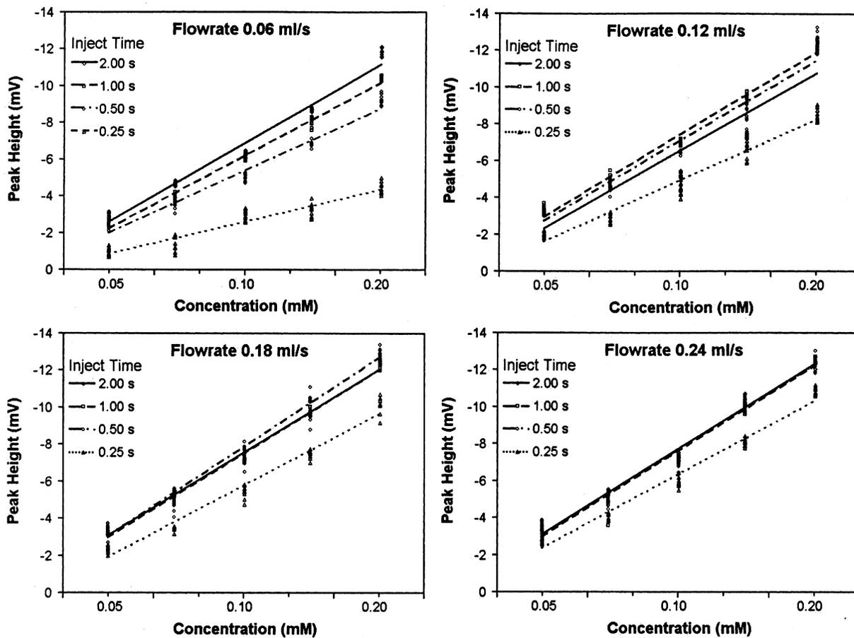
Fig. 5. Signal peak height vs. concentration of nitrate for different flowrates (0.06, 0.12, 0.18, and 0.24 ml/s) and injection times (0.25, 0.5, 1.0, and 2.0 s) with 2.0 s washout time.
