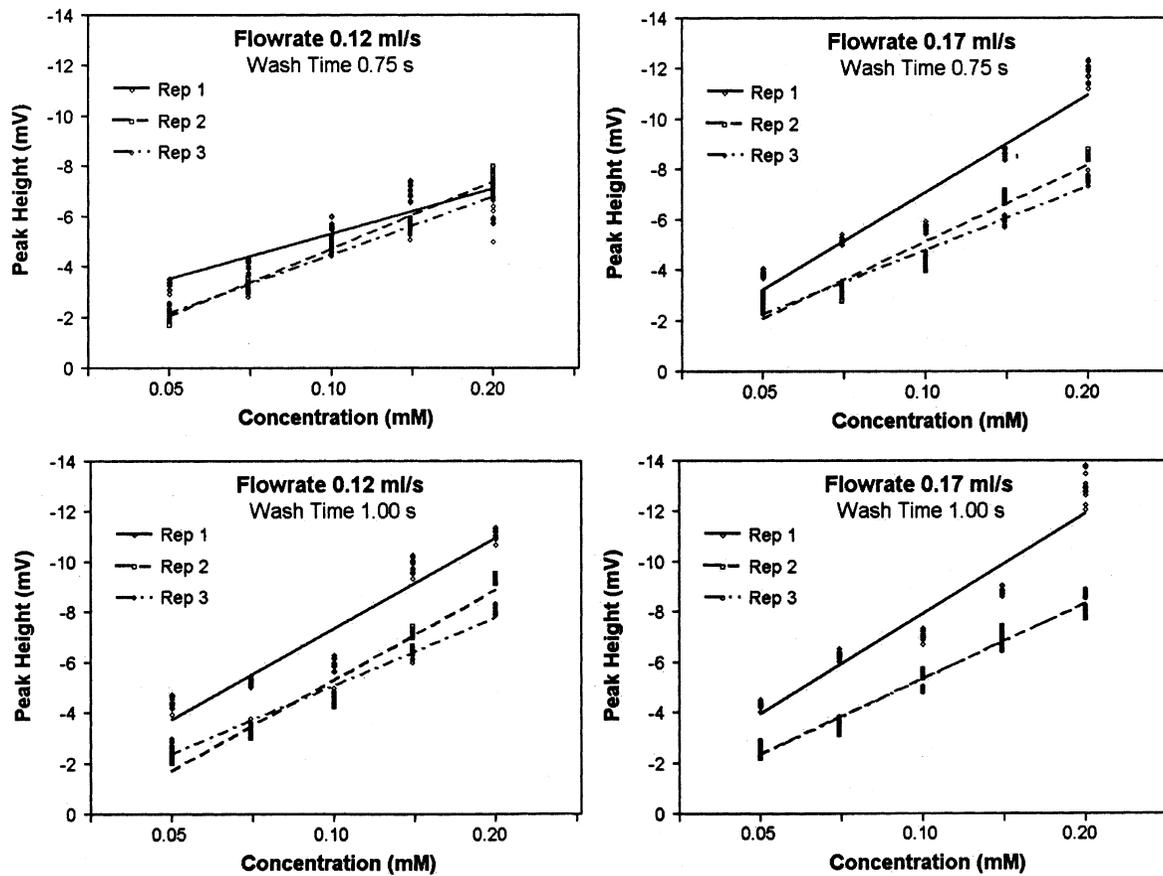
Fig. 6. Signal peak height vs. concentration of nitrate for two flowrates (0.12, and 0.17 ml/s) and washout times (0.75 and 1.0 s) with 0.5 s injection time.
