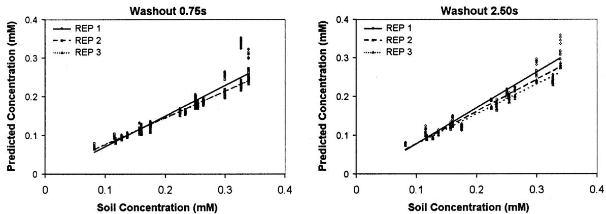
Fig. 7. Predicted vs. actual soil nitrate concentration for manually extracted solutions with 0.75 s (left) and 2.5 s (right) washout time.
