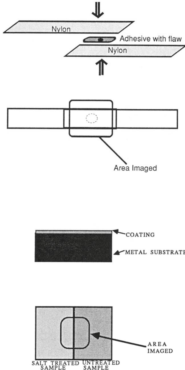
Figure 4. Schematic diagram of the nylon or composite and paint panel samples.
