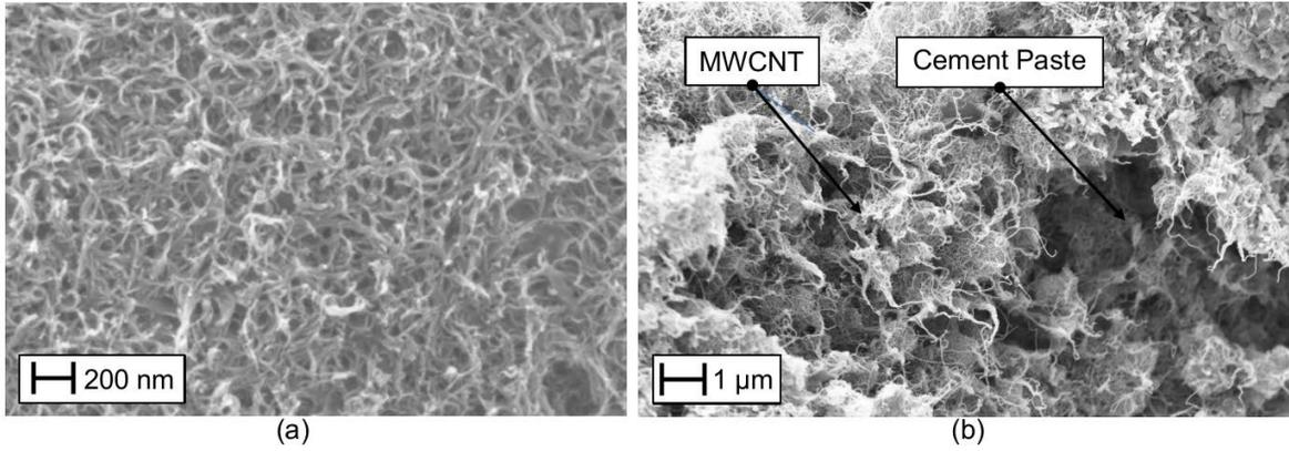
**FIGURE 2.** Scanning electron micrographs of water solution with MWCNT (a) cement paste with MWCNT (b).
