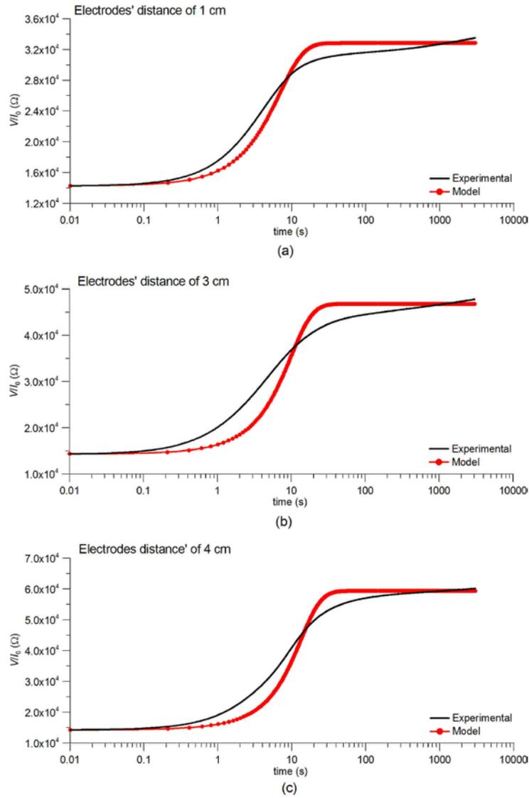
**FIGURE 6.** Comparison between experimental results and analytical predictions for the step response of CNTCSs with varying distances between the active electrodes: 1 cm (a); 3 cm (b); and 4 cm (c).
