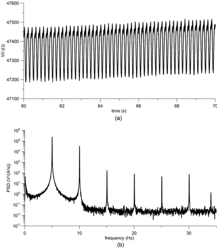
**FIGURE 7.** Variation of apparent resistance (a) and its PSD (b) under 5 Hz sinusoidal axial loading ( $1 \pm 0.5$  kN) for a distance between the electrodes of 3 cm.
