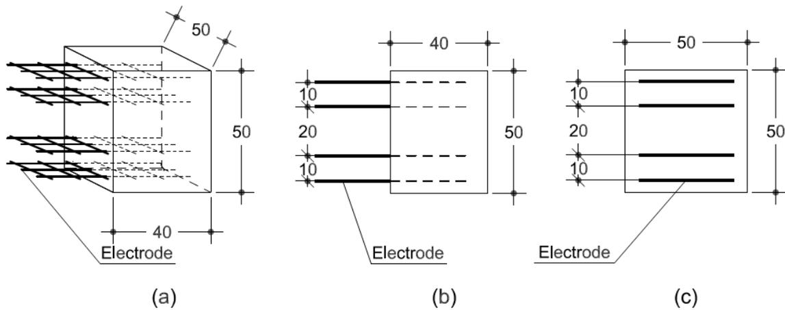
**FIGURE 3.** Sketch and dimensions (in mm) of the Carbon Nanotube Cement-based Sensor: axonometric view (a), side view (b), and front view (c).
