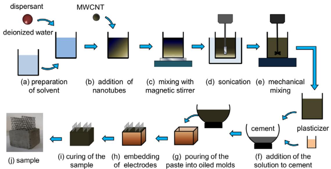
**FIGURE 1.** Preparation scheme of CNTCS with embedded steel net electrodes.
