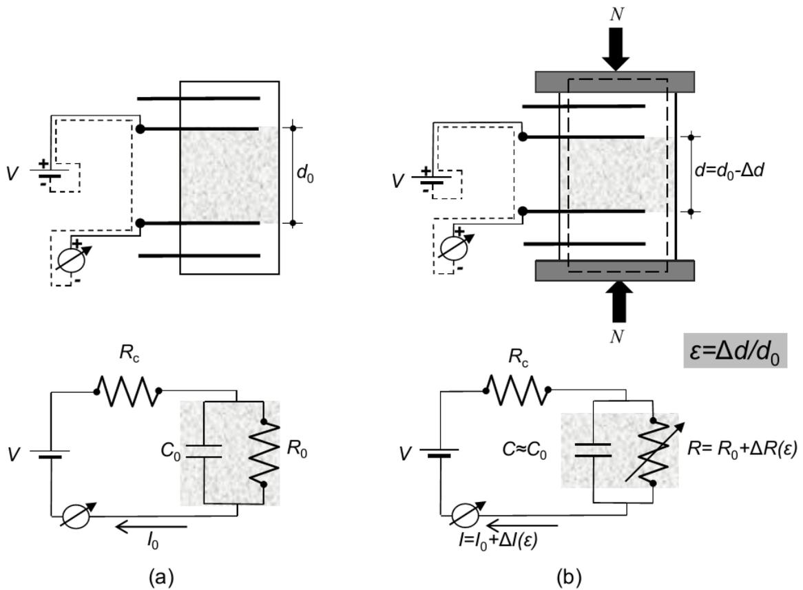
**FIGURE 4.** Schematic of the proposed electromechanical model of a CNTCS: unloaded (a) and loaded samples (b).
