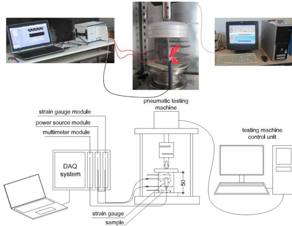
**FIGURE 5.** Experimental setup. From left to right, data acquisition system, sample placed in the axial pneumatic testing machine, and testing machine control unit.
