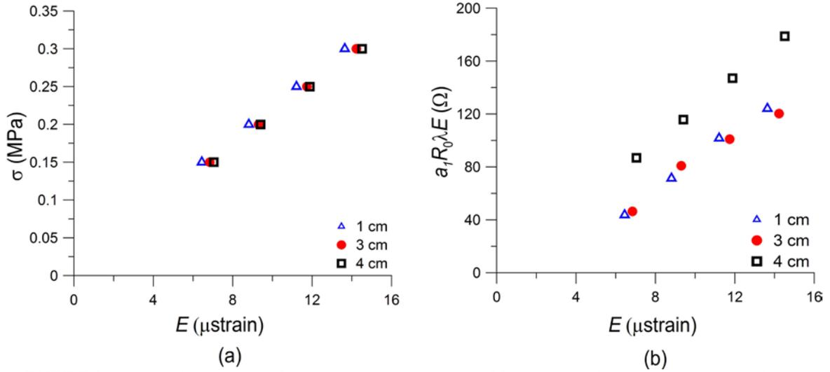
**FIGURE 8.** Stress-strain behaviour of the sensor (a) and amplitude of first harmonic in Eq. (8) versus the strain amplitude (b).
