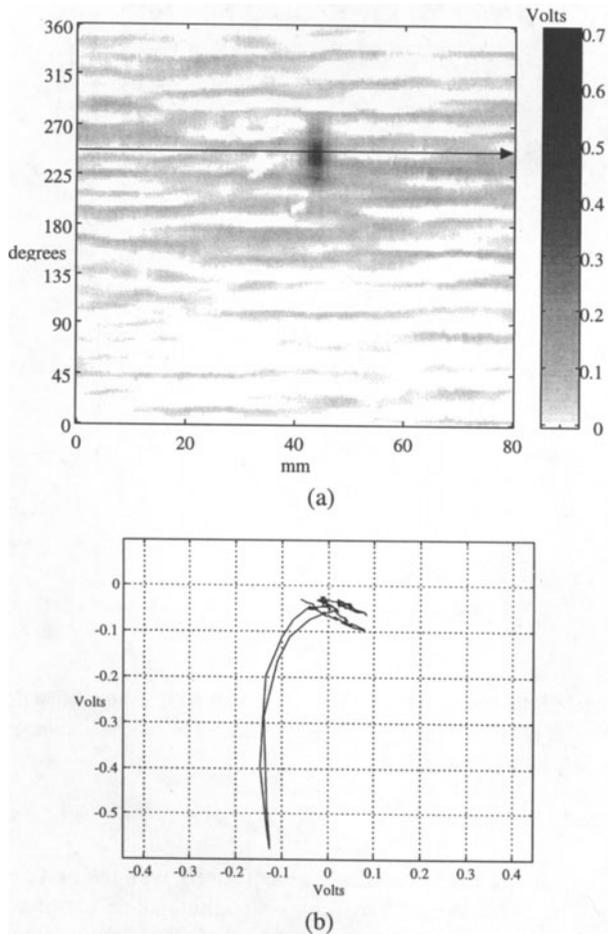
Figure 6. Inspection of the transversal slot (0.1-mm wide, 45° range, 40% depth) with the MRPC (2.6-mm diameter) at frequency,  $F$ , = of 240 kHz (a) cartography of the eddy currents signal module (b) Lissajous figure extracted following the arrow.
