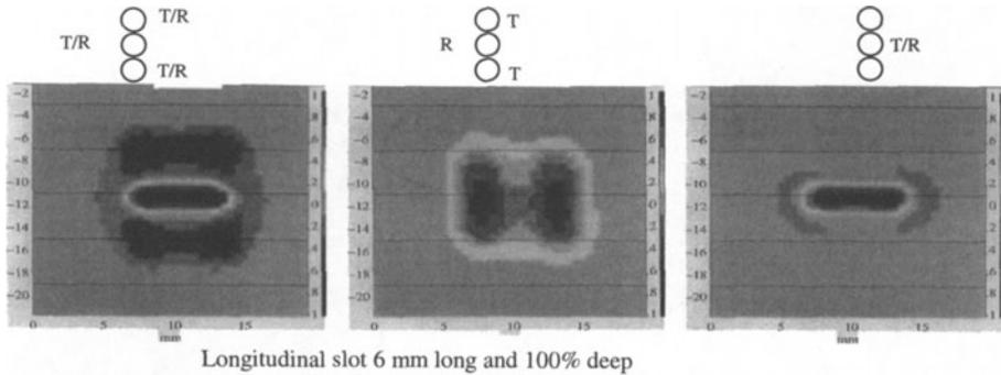
Figure 2. Influence zones of the three configurations on a longitudinal defect.
