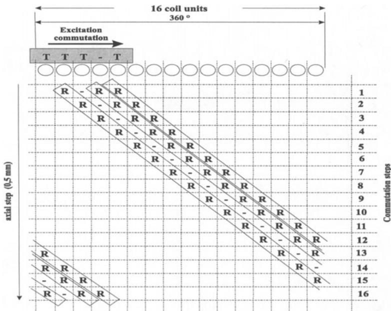
Figure 3. Mask switching sequence for 16 detector units.
