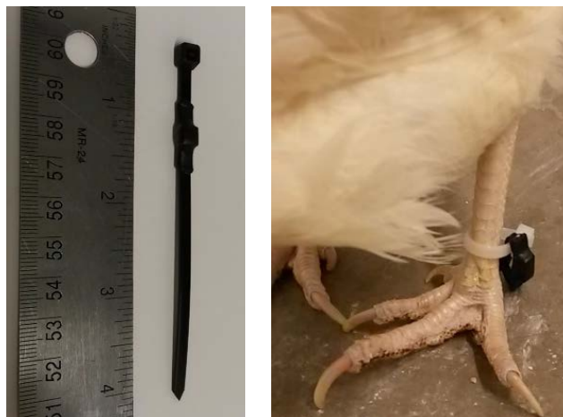
Figure 2. The RFID transponder (left) and its attachment to a hen's leg (right).
