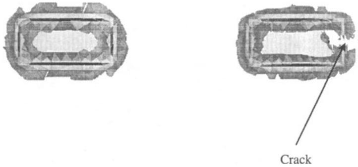
Fig. 4. Finite element results of the induced eddy current density in an electrically conductive sample with and without a crack present.
