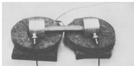
RUBBER CHANNEL FILLED WITH CURING RESIN TO FORM ACOUSTIC WAVEGUIDE BETWEEN ACOUSTIC TRANSMITTER AND RECEIVER.
