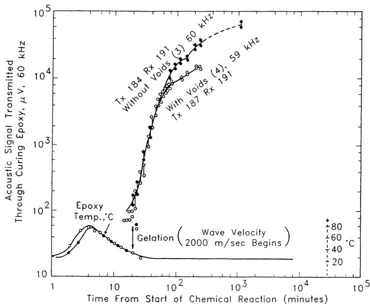
Figure 5. Changes in acoustic signals transmitted through curing epoxy with and without artificial voids.
