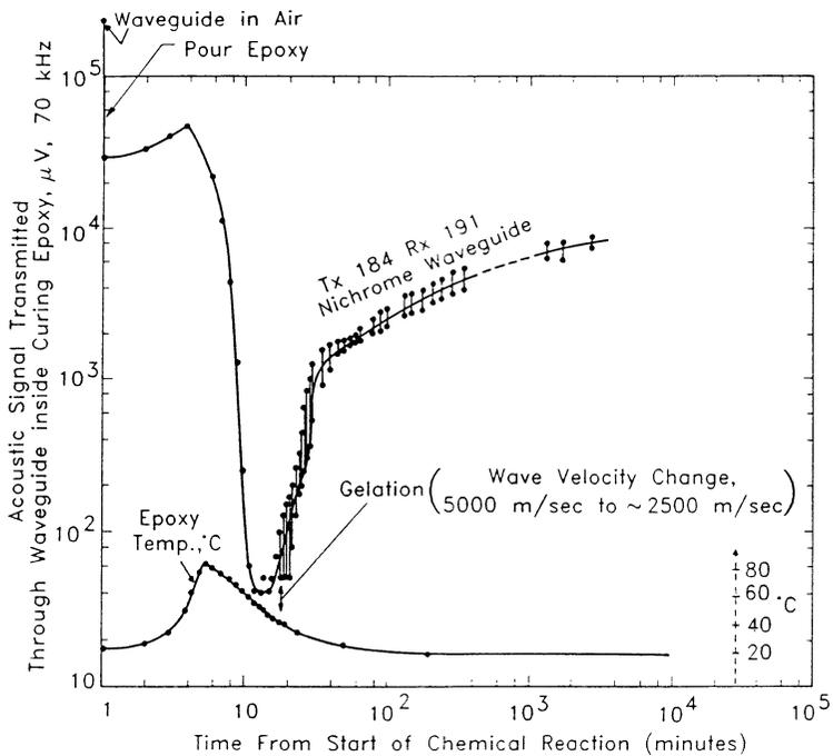
Figure 7. Changes in acoustic signals transmitted through Nichrome waveguide inside curing epoxy.
