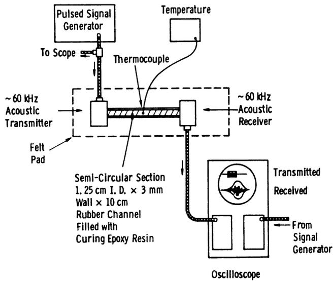
Figure 1. Schematic of experimental apparatus for determining the acoustical properties of curing resin filled with hollow spheres.
