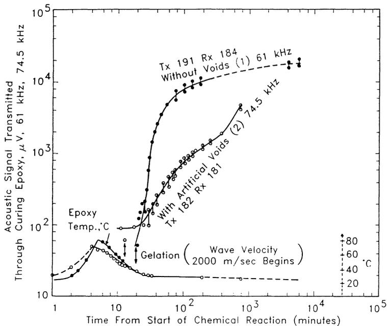
Figure 4. Changes in the acoustic signals transmitted through curing epoxy with and without artificial voids.
