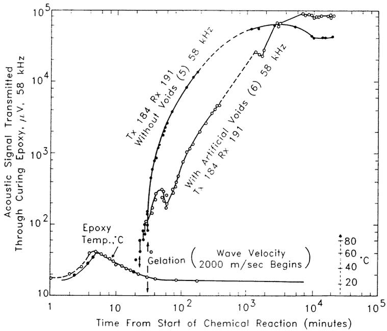
Figure 6. Changes in the acoustic signals transmitted through curing epoxy with and without artificial voids.
