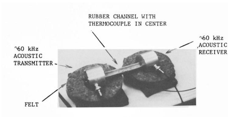
EMPTY RUBBER CHANNEL CONNECTED BETWEEN ACOUSTIC TRANSMITTER AND RECEIVER.
