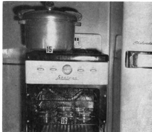
**Fig. C:** Pressure cooker (15), oven used for sterilizing Petri dishes (16).
