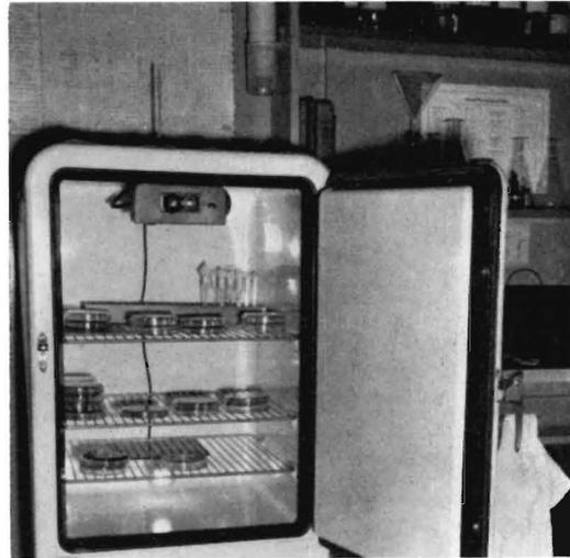
Fig. D: Incubator (converted refrigerator).
