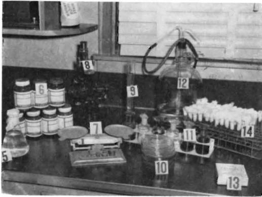
**Fig. B:** Erlenmyer Flasks (5), Dehydrated Media (6), Balances (7), Microscope (8), Graduate cylinder (9), Petri dishes (10), Stains and containers (11), Distilled water (12), Slides (13), Test tubes and rack (14).
