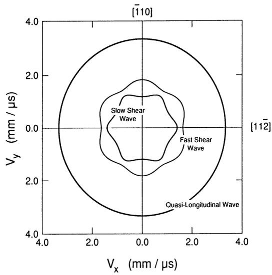
Fig. 2a The phase velocity in the (111) plane of CdTe.
