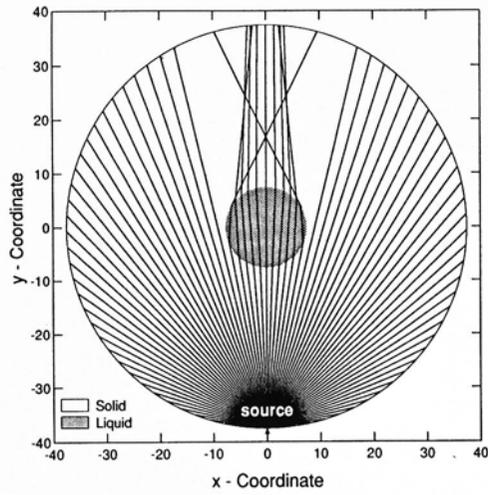
Fig. 4 The calculated ray paths for a [001] crystal cylinder,  $R = 37.5$  mm,  $r = 7.5$  mm.
