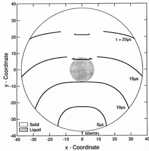
Fig. 5 The quasilongitudinal wave fronts for a [001] crystal cylinder,  $R = 37.5$  mm,  $r = 7.5$  mm.
