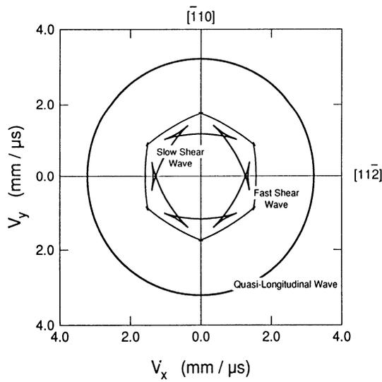
Fig. 2b The group velocity in the (111) plane of CdTe.
