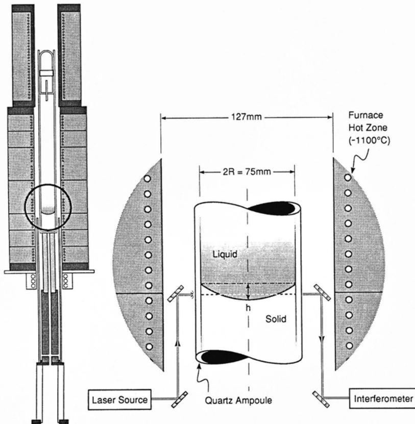
Fig. 1 A schematic arrangement of ultrasonic sensing in a vertical Bridgman furnace.
