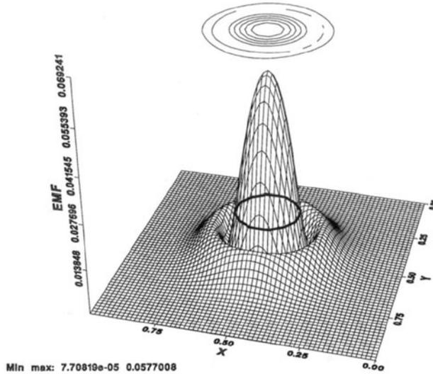
Fig. 4. Signals transmitted through a multi-layer composite of 36 alternating +45/-45 degree layers. Zero-to-peak magnitude is approximately  $5.8 \times 10^{-2}$  [EMF]. Orbits represent equi-potential contours.
