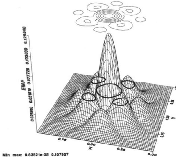
Fig. 6. Calculation of EMF magnitude transmitted through a 36-layer sample having four groups of nine layers. The four groups are oriented  $+45/-45/+45/-45$  degrees. The peak EMF magnitude is approximately  $1.1 \times 10^{-1}$ .
