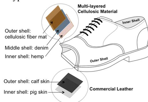
Figure 1. Material structures.
