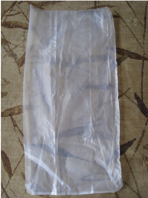
Figure 4. PICS 80-µm polyethelene inner bag.
