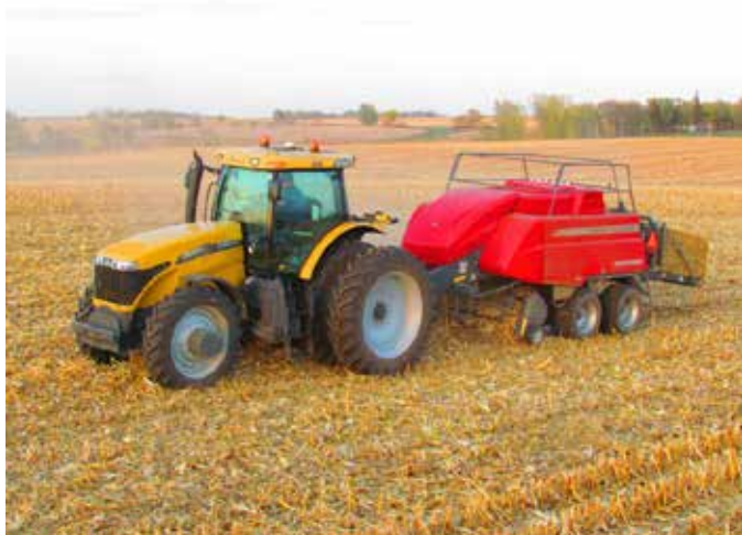
Figure 3. Three foot by four foot large square baler used in corn stover production.
