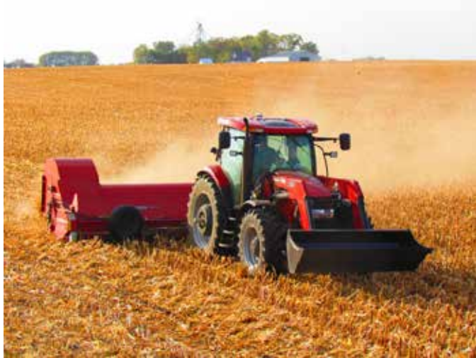
Figure 2. Side discharge windrowing stalk chopper forming a corn stover windrow.
