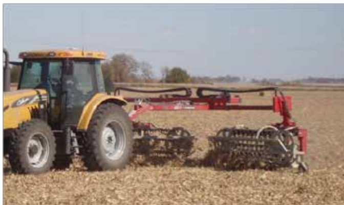
Figure 1. Hydraulically powered bar rake forming a corn stover windrow.
