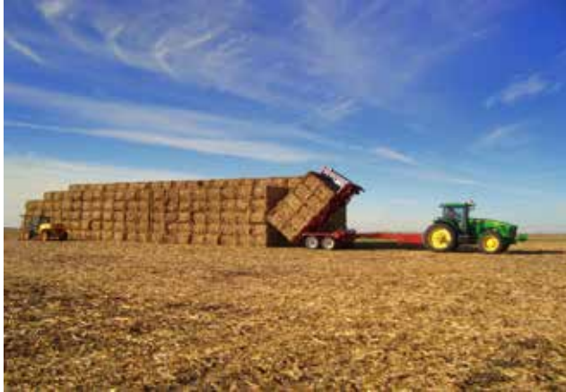
Figure 6. Large square bale collection wagon used to collect bales and create a field stack.
