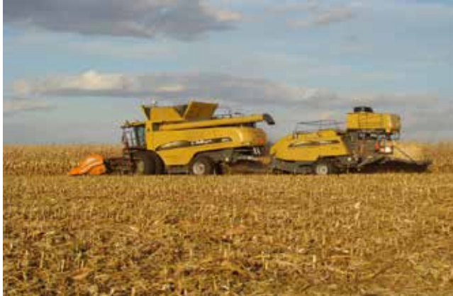
Figure 4. AGCO single pass combine producing corn stover bales simultaneously with corn grain harvest.
