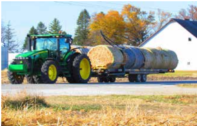
Figure 5. Round bale collection wagon used to move round bales from a field to a storage facility.
