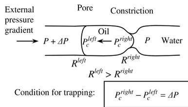
**Figure 1.** Organic-ganglion flow through a constricted pore under the effect of external pressure difference  $\Delta P$ .  $R^{left}$  and  $R^{right}$  are the radii of the left and the right menisci, respectively. The ganglion is trapped when the condition in the box is satisfied.
