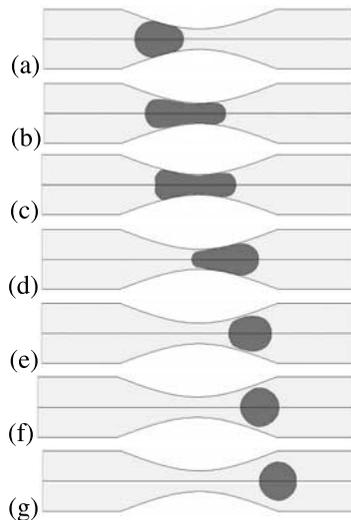
**Figure 6.** Numerical simulation of the organic-ganglion mobilization by vibrations of the wall. Snapshots are made at 0.0, 0.025, 0.050, 0.075, 0.100, 0.125, and 0.150 sec (a–g, respectively) after the vibrations were turned on; (a) corresponds to the initial entrapped configuration.
