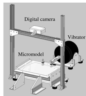
**Figure 3.** Sketch of the experimental set-up.
