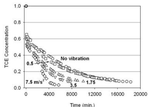
**Figure 5.** Concentration of TCE as a function of time. The effect of vibration with different acceleration amplitudes is shown, at a constant frequency of 30 Hz.
