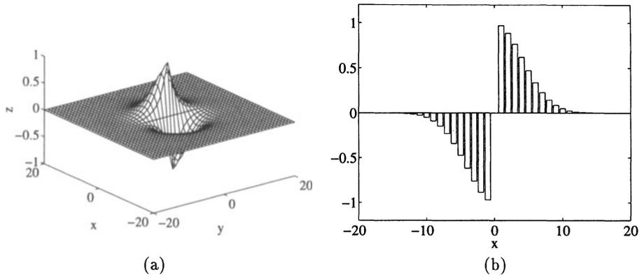
Figure 2: (a) The directional difference mask in  $x$ -direction of the GWIMV and (b) The cross section of the difference mask at  $y = 0$
