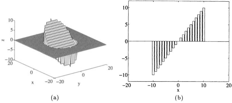
Figure 1: (a) The directional difference mask in  $x$ -direction of the IMV and (b) The cross section of the difference mask at  $y = 0$
