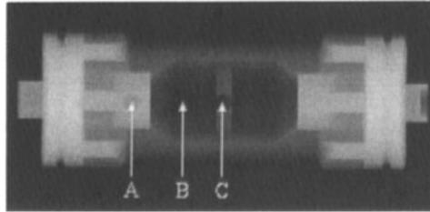
Figure 7: The simulated x-ray image of the object with spherical flaws with diameter varied from 1 to 5 mm. in 3 locations.
