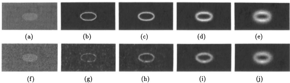
Figure 4: (a) The original image without noise and edge images with (b)  $\sigma = 1$ , (c)  $\sigma = 2$ , (d)  $\sigma = 4.2$ , (e)  $\sigma = 8$ . (f) The noisy image degraded by the additive Gaussian noise with  $\text{SNR} = 2$ , and edge images with (g)  $\sigma = 1$ , (h)  $\sigma = 2$ , (i)  $\sigma = 4.2$ , (j)  $\sigma = 8$
