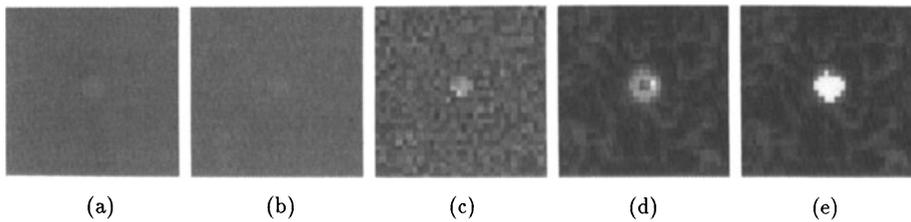
Figure 6: (a) The original flaw image. (b) The noisy flaw image. (c) The histogram stretching image of Figure b. (d) The optimum edge image. (e) The enhanced flaw image.
