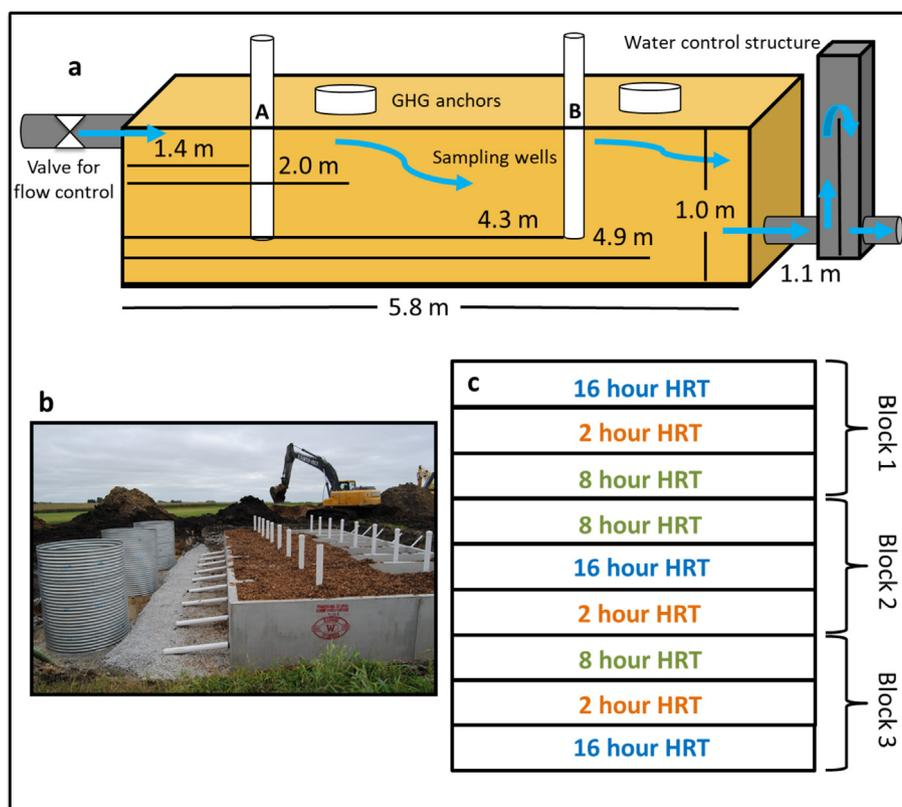
Fig. 1. (a) Bioreactor layout with sampling locations, distances from the inlet, and illustrated flow path. (b) Photo of installation before control structures were installed at the outlet. (c) Randomized complete block design for hydraulic residence times (HRTs) of pilot scale bioreactors. Bioreactors were blocked by inlet pipe.
