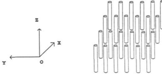
Figure 1. A 3-D schematic of the right circular cylinders of polyethylene in a polycrystalline iron background in a periodic 2-D array. The cylinders form a square lattice, with sides,  $L_T = 0.06$  mm for transverse elastic waves, and  $L_L = 0.7$  mm for longitudinal elastic waves. The coordinate system is shown.
