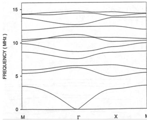
Figure 3. The dispersion relations,  $\omega_{\vec{k}n}$  vs  $\vec{k}$  for Polyethylene cylinders in a square lattice of iron with filling factor  $f_0 = 0.7$  for longitudinal elastic waves,  $a = 0.60$  mm.
