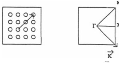
Figure 2 The top view of the direct space lattice with separation  $\vec{R}$  between lattice sites on the left. The vector shows the location of the second neighbor. The first Brillouin zone for the square lattice on the right. The high symmetry  $\vec{k}$  points are  $X(1, 0, 0)$ ,  $\Gamma(0, 0, 0)$ , and  $M(1, 1, 0)$ .
