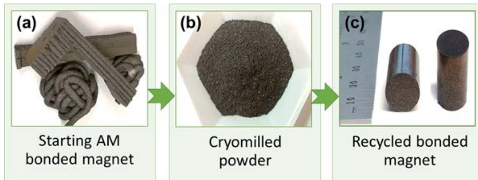
Fig. 1. (a) Starting AM bonded magnets (65 vol.% Nd-Fe-B in nylon), (b) cryomilled powder, and (c) recycled bonded magnets.
