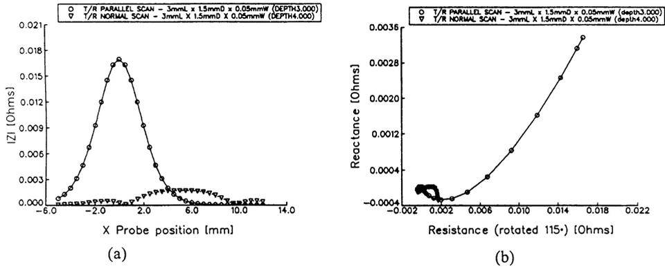
Figure 2: Comparison of signal outputs shows different results due to normal and parallel scan orientations. The magnitudes are shown in (a), and the impedance plane trajectories are shown in (b).
