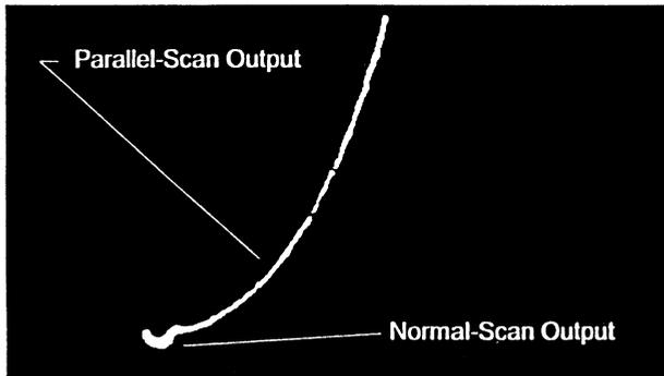
Figure 3: Impedance plane trajectories of two different scan orientations are shown, based on laboratory test results at 100 kHz.
