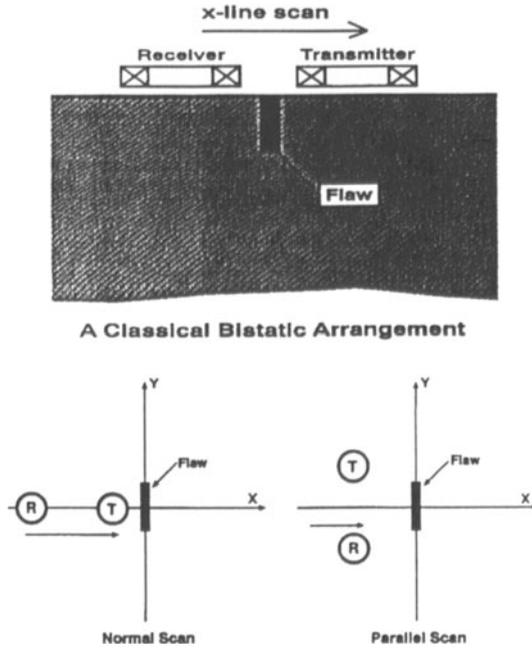
Figure 1: A bistatic arrangement of a typical transmit-receive coil configuration is shown along with the typical scan orientations.
